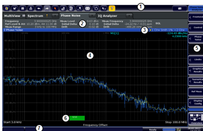
Fig. 2-1: Screen layout of the phase noise measurement application
